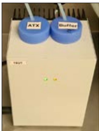
Position of ATX tube in the cooling block
