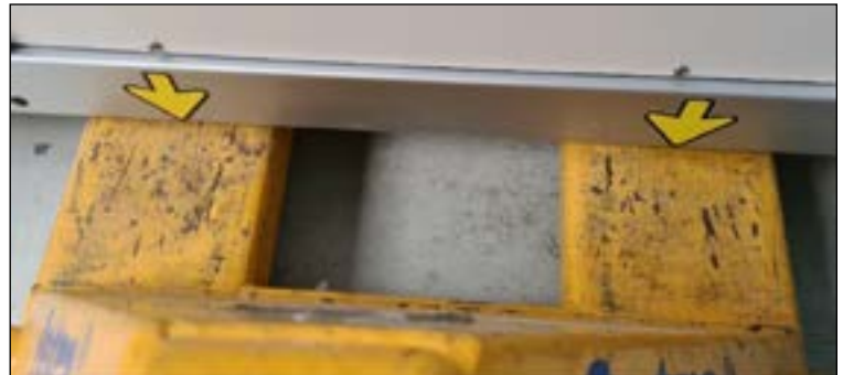
Fork placement when lifting the Autosampler III
