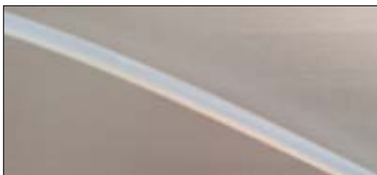
Correct tubing (little to no air bubbles)
