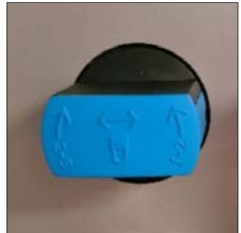
Compressed air valve in open state
