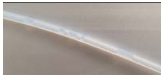
Incorrect tubing (significant amount of air)
