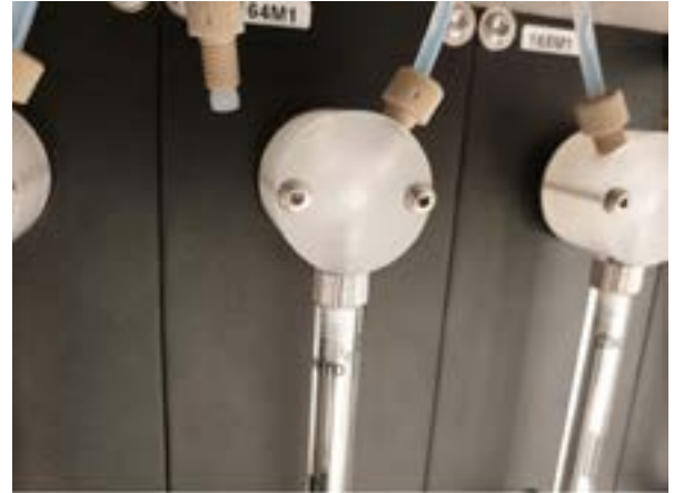
Picture of what tubing to detach from the pump when using ethanol
