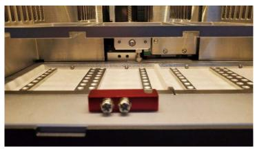
b. Install the Fixing Block.
