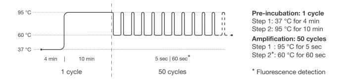
For some real-time PCR instruments the probe quencher as well as the use of a passive reference dye must be specified. This kit contains probes with a non-fluorescent "dark" quencher and no passive reference dye.
