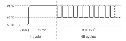
Pre-incubation: 1 cycle Step 1: 50 °C for 2 min Step 2: 95 °C for 10 min Amplification: 45 cycles Step 1: 95 °C for 15 s Step 2\*: 60 °C for 60 s
