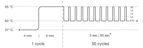
Pre-incubation: 1 cycle Step 1: 37 °C for 4 min Step 2: 95 °C for 5 min Amplification: 50 cycles Step 1: 95 °C for 5 sec Step 2\*: 60 °C for 60 sec
